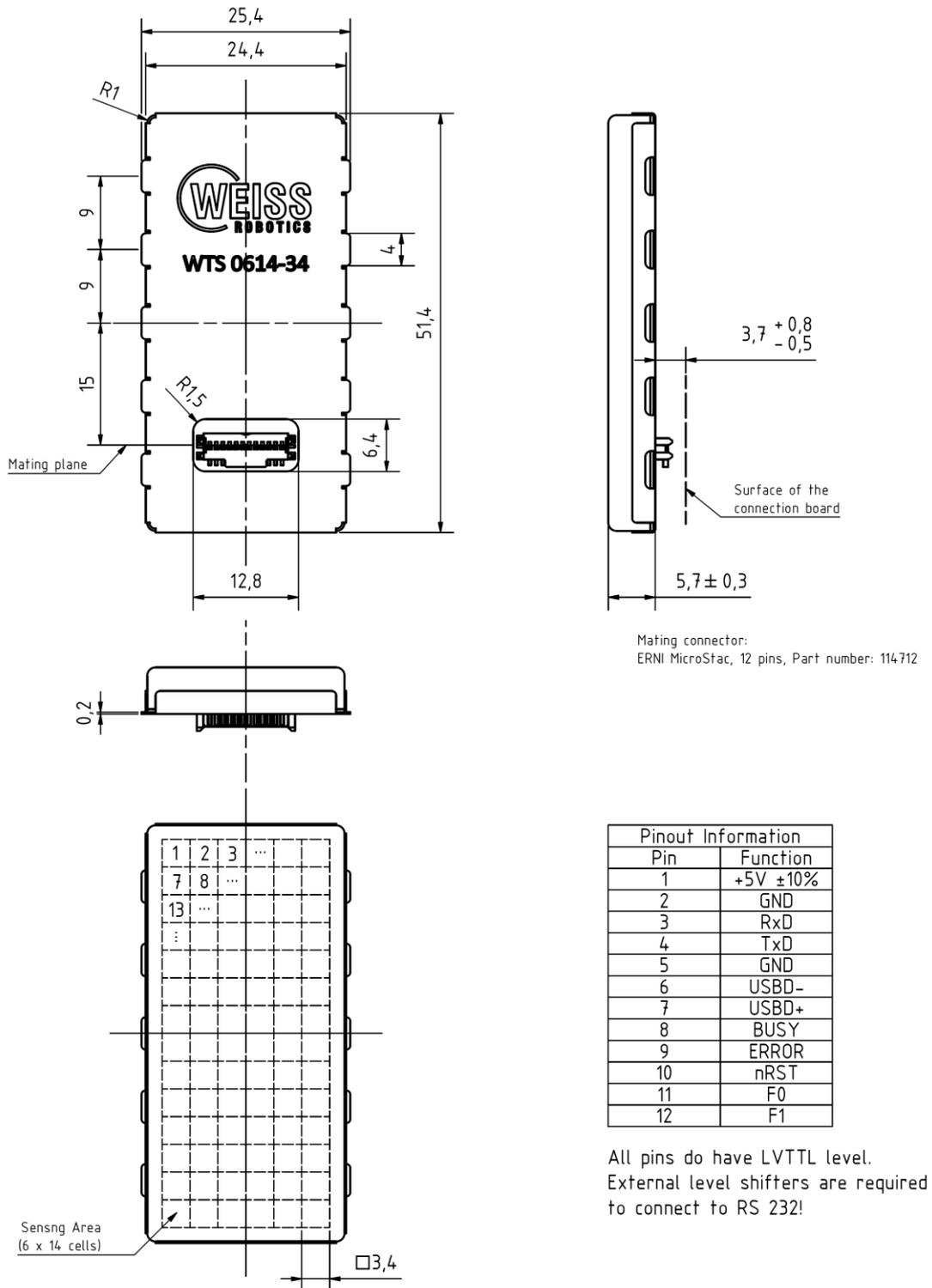
Fig. 3: Mechanical Dimensions
